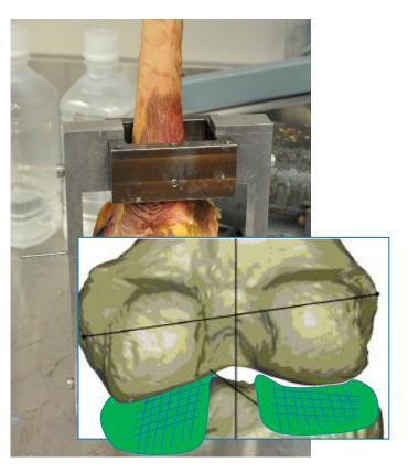
3. Insert Tekscan sensor – secured to ACL and posterior capsule
