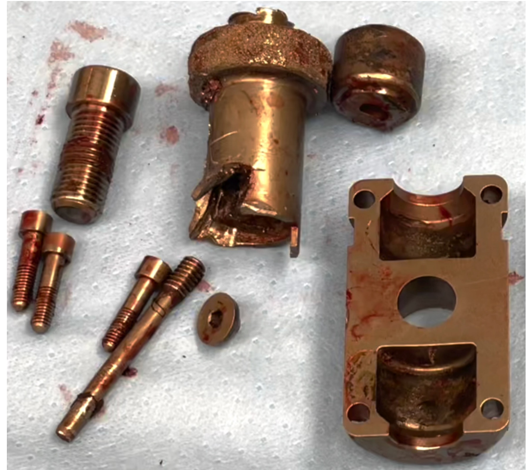
Figure 4. Broken proximal diaphyseal connector with excessive wear of locking collar.
