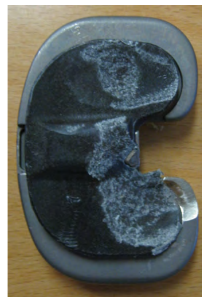
02 Worn carbon fiber reinforced polyethylene
