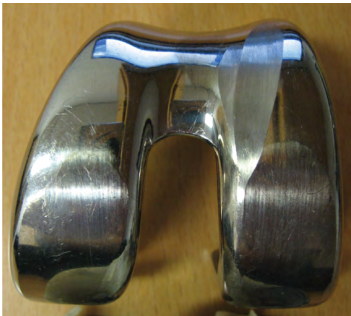
03 Titanium femoral component with marked scoring
